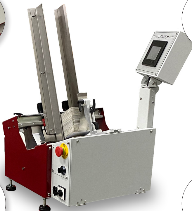
High quality structure, with PLC and encoder.
