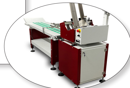
Base and conveyor for product separation (O)
